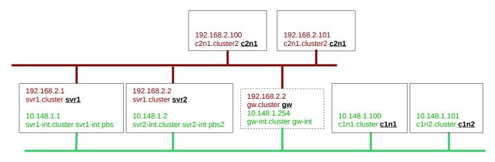
The same solutions used in the previous section apply here, except that the second solution cannot be used on its own (since the PBS leaf address for the server and PBS\_SERVER cannot be on two networks at the same time).
