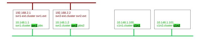
Here all hostnames (marked in colour) resolve to an IP address that is on the network that PBSPro is meant to use.
